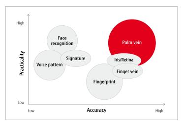
Fujitsu's PalmSecure technology uses a biometric pattern inside the body. It is certified by ISO and approved by the German Ministry of IT Security. The following table ranks biometric methods on their False Acceptance Rate (FAR) and False Rejection Rate (FRR). These indicators define the security level of a biometric system (FAR) and the usability of a biometric system (FRR).
