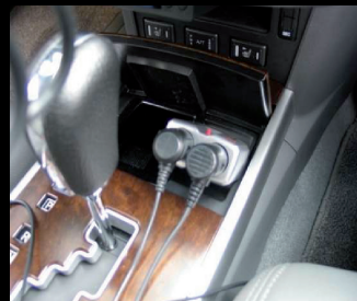
Connect the JANUS V2 power cable to the cigar lighter
